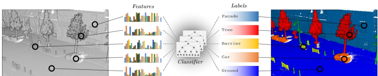
Figure 23. Standard pointwise classification framework. A set of features is computed for every point of the scene and a classifier is used to label each point independently.
