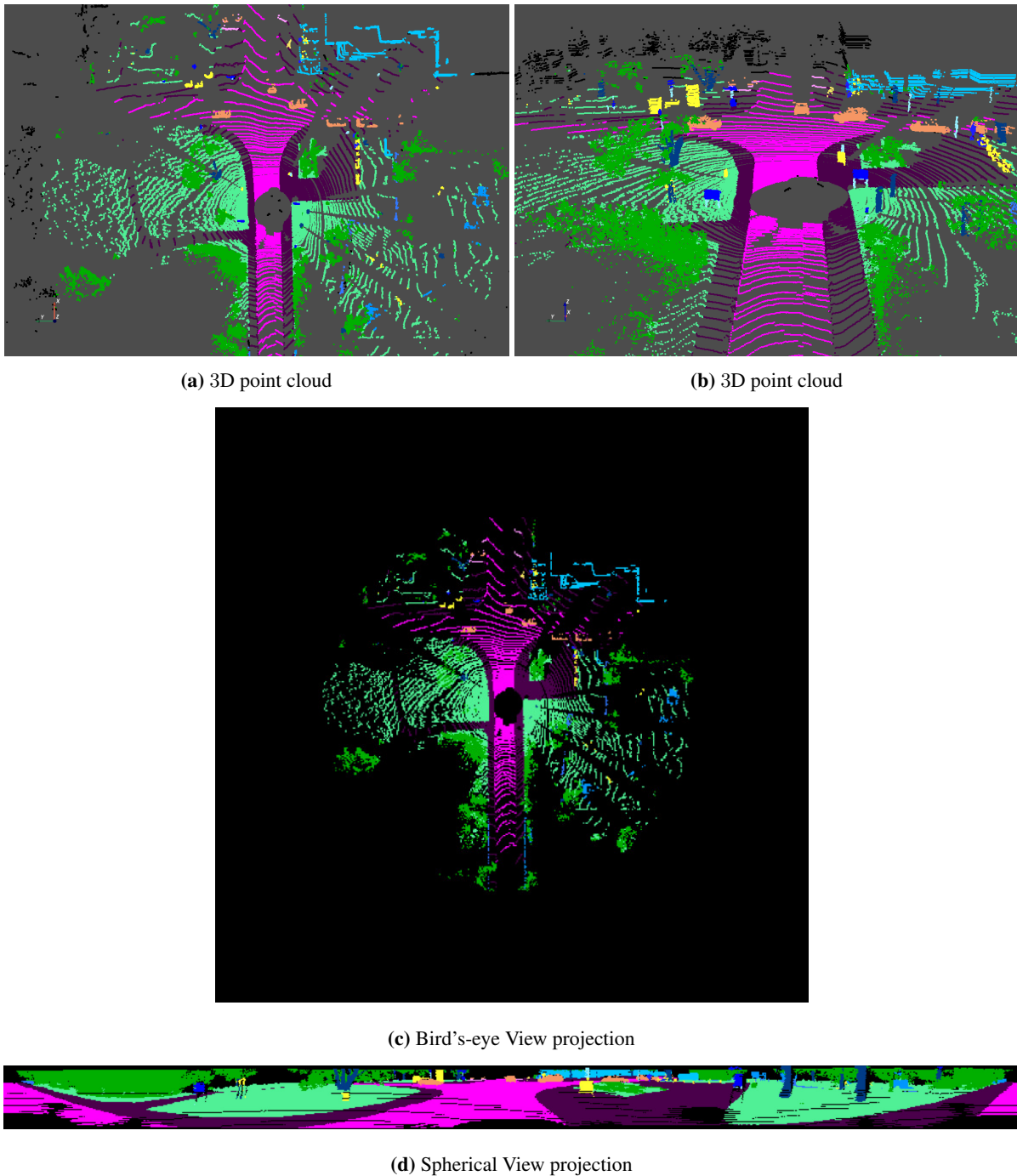
Figure 2.7 An example of projection of a point cloud onto images. (a, b) Two views of the same 3D point cloud. (c) Image obtained after a Bird's-eye View projection, (d) Image obtained after a Spherical View projection. Some pixels are black because no point falls in.
