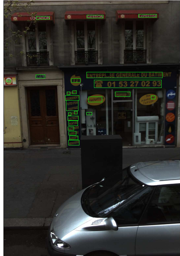
Fig. 22 ITOWNS image result of our text detection. All the boxes of detected texts have been superimposed in green color.
