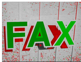
Fig. 13 Result of our classification process on the FAX image: regions from figure 9 are classified as text (green regions) or not text (red regions).
