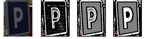
Fig. 3. From left to right: 1. Original image, 2. Binarization (function s from eq. 6), 3. Homogeneity constraint (eq. 7), 4. Filling in small homogeneous regions.
